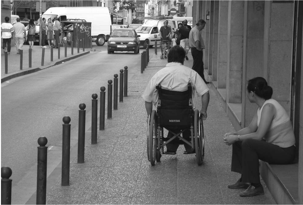
Figure 7.6 Narrow footways impede accessibility.
